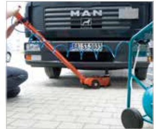
▶ Intuitive safety rotary button control with compressor coupling
